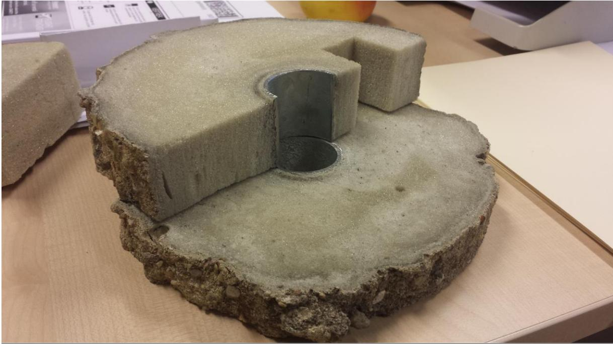
**\*Cross cut Large Kit with a metal post, clearly showing the penetration into the ground**
